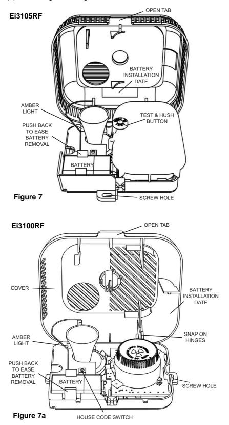
1. Pull cover open at tab. Remove cover from base by separating at rear snap-in hinges by rotating cover backwards.
